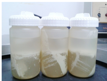
Figure 2 The separation of coconut milk after using refrigerated centrifugation. At 15, 20 and 26 °C (15 and 20 °C couldn't provide VCO separation and Re-centrifugation at 26 °C)
