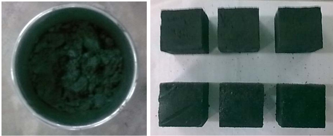
Figure 2 Fresh and Hardened Geopolymer Mortar
