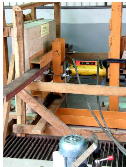
Figure 4 Installation of loading frame
