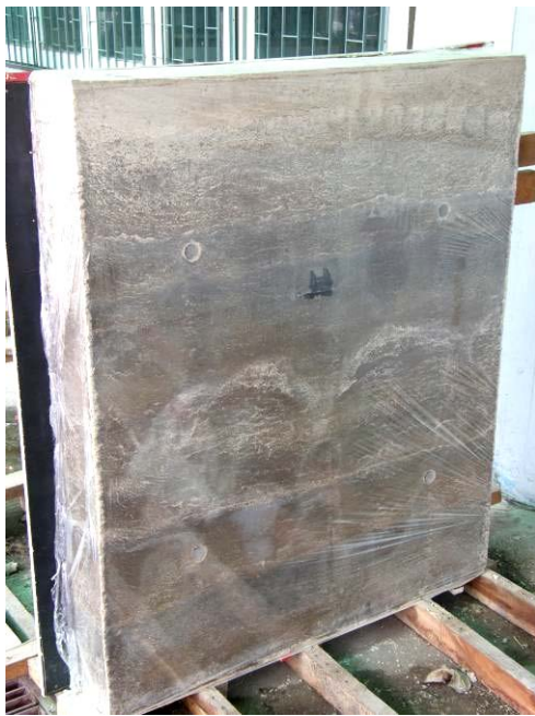
Figure 7 Cement stabilized rammed earth wall
