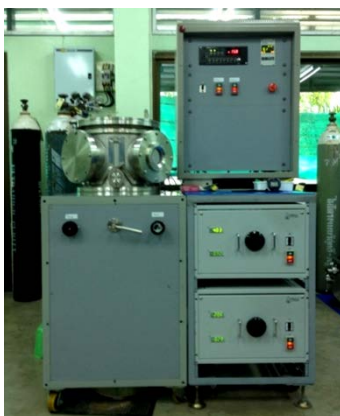
Figure 1 Features and diagram of the DC co-unbalanced magnetron sputtering system
