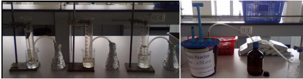
Figure 2 Experimental set CH_4 and Laboratory scale experiments for biogas production by anaerobic digestion process
