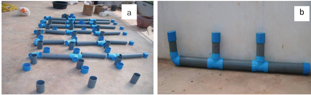
Figure 1 Pieces of PVC pipes to construct the compost pile simulator before assemble (a) and after assemble (b).
