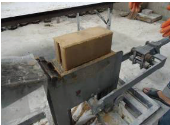
Figure 3 Kaolin Interlocking blocks 25 cm long, 10 cm thick and 10 cm high.
